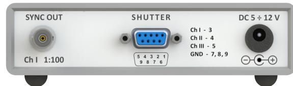
**SHUTTER** (D-SUB) connector is used for HV pulses output. Connector pinout:
